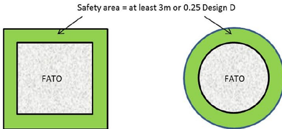
Figure 3-1. FATO and associated safety area
