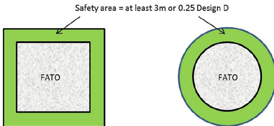
Figure 3-1. FATO and associated safety area
